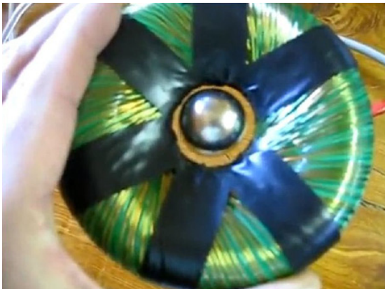
Fig 5. Levitating magnet above a Rodin coil [7]
